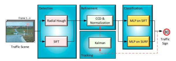
Figure 11. An example of a TSDR system includes tracking process based on Kalman filter [81].
