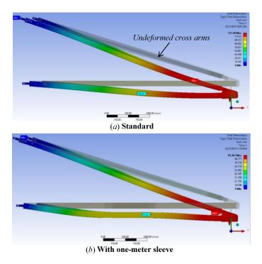
**Figure 3.** Comparison of deformation between (*a*) the standard cross arm without sleeve and (*b*) the cross arm with one-meter sleeve installed, upon being subjected to statics loading.
