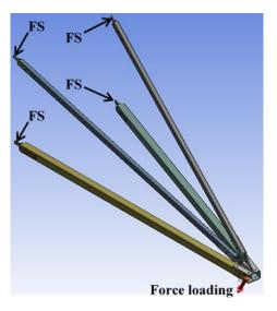
**Figure 2.** Summary of boundary conditions that being applied on the cross-arms numerical model. The abbreviation "FS" denotes to fixed support boundary condition that applied on the cross arms hinges.
