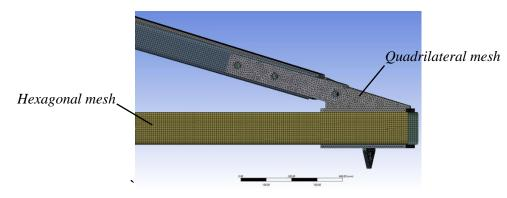
Figure 1. The adaptive hybrid mesh that being implemneted on the cross arms numerical model.
