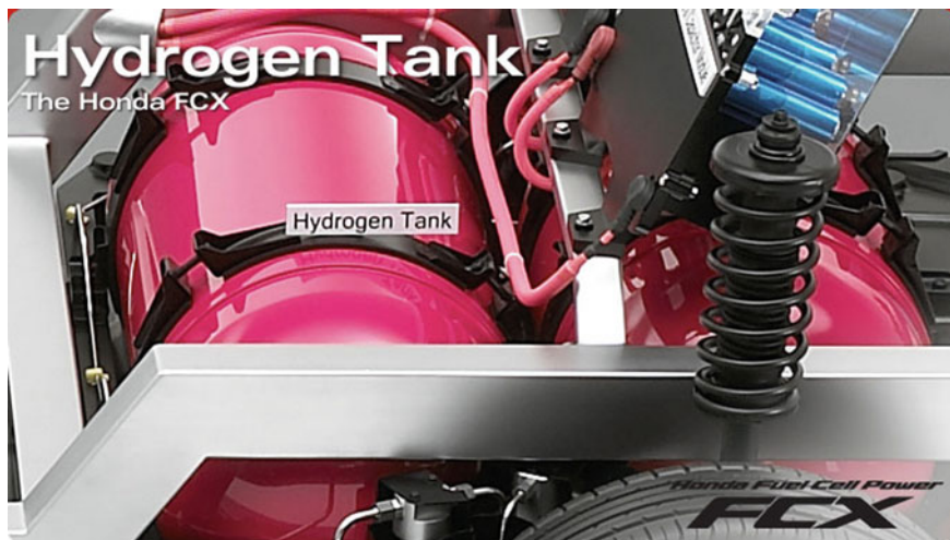
Fig. 5.3 Two 350 bar high-pressure hydrogen tanks from the Honda FCX Clarity (Source http://world.honda.com/FuelCell/FCX/tank/ )
