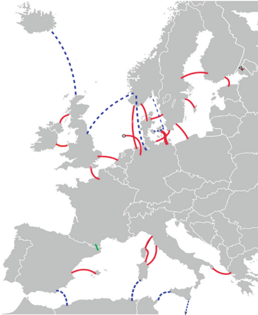
Fig. 3.2 Early high voltage DC connections. Solid lines show existing links and those under construction dashed and lines show proposed links (Source http://en.wikipedia.org/wiki/High-voltage_direct_current )
