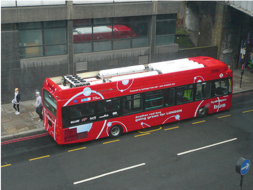
Fig. 8.21 An elevated view of London's first hydrogen fuel cell bus showing the six roof-mounted hydrogen fuel tanks (Source http://en.wikipedia.org/wiki/Fuel_cell_bus )
