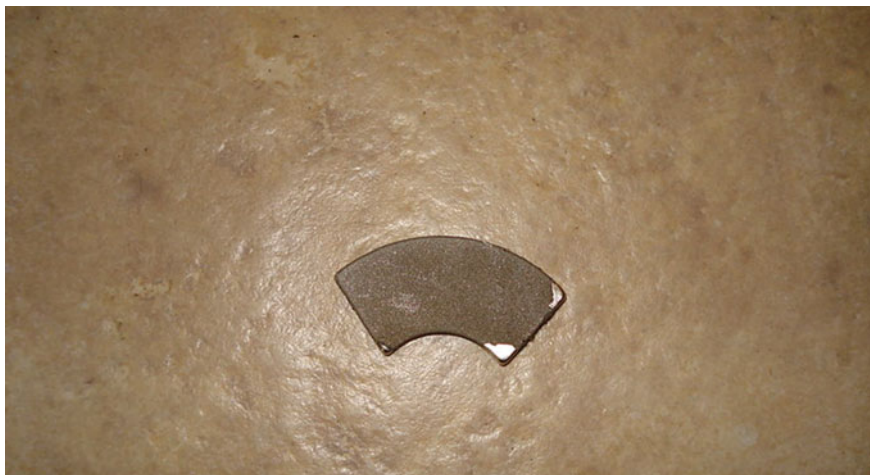
Fig. 10.6 Neodymium magnet with nickel plate mostly removed (Source http://upload.wikimedia.org/wikipedia/commons/d/de/Neodymium_magnet_-_19-11-2010.JPG )
