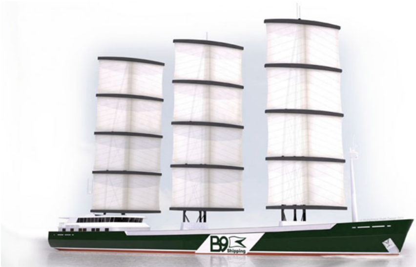
Fig. 9.13 B9 Shipping’s sailing cargo ships would feature a Dyna-rig sail system (Reproduced with kind permission of B9 shipping/HYD)
