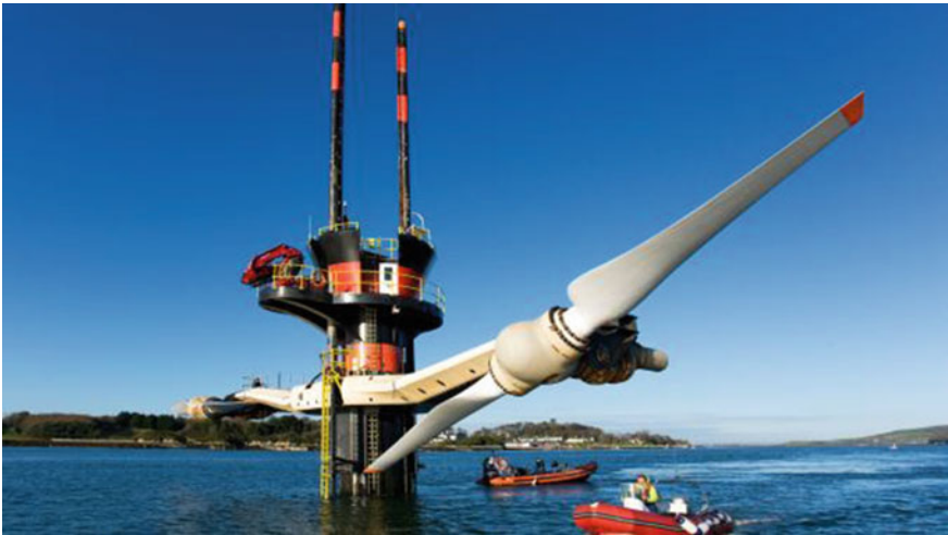
Fig. 4.8 Commercial marine turbine with its rotors raised (Reproduced with kind permission Marine Current Turbines Ltd)
