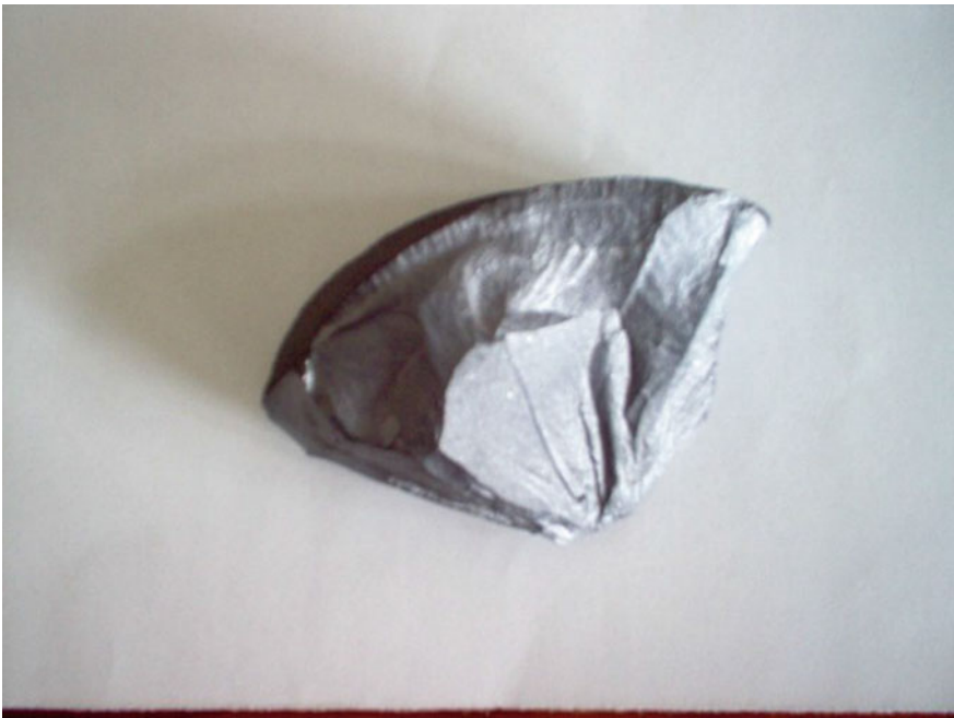
Fig. 10.4 Polycrystalline silicon used to produce silicon monocrystals (Source http://en.wikipedia.org/wiki/Polycrystalline_silicon )
