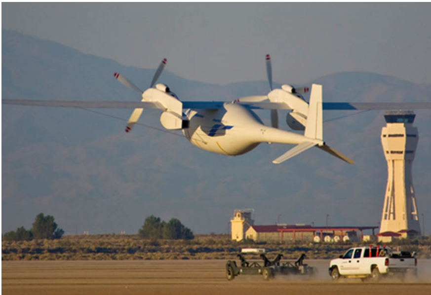
Fig. 9.6 Phantom Eye taking off from launch trolley (Source http://phys.ofdrg/news/2012-06-phantom-eye-liquid-hydrogen-powered-unmanned.html ) (Reproduced with kind permission of Boeing)
