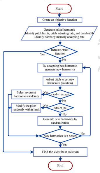
Fig. 11. Basic structure of HSA.
