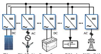
PV array Wind Turbine Energy Syorage DC load Utility Grid
