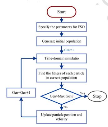
Fig. 14. Flowchart of the PSO algorithm.
