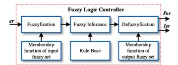
Fig. 10. General block diagram of fuzzy logic controller.
