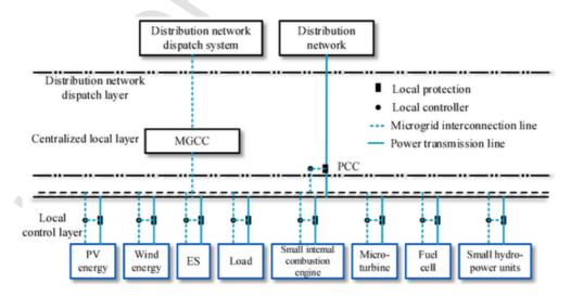
Fig. 4. Composition and structure of MG.
